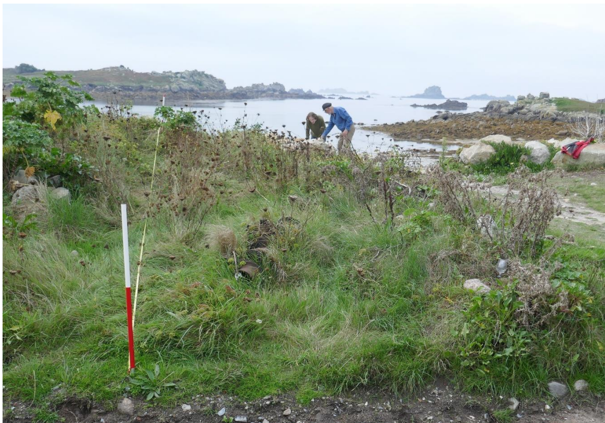
Fig 61 Surveying the Czar shed, by measuring off at right angles from a baseline tape. This method allows rapid accurate survey of smaller sites with minimal equipment.
