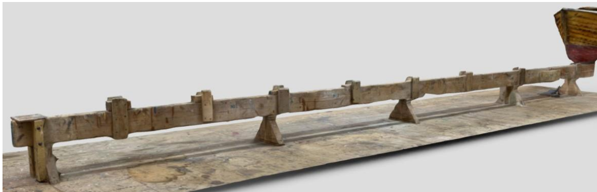
Fig 25 Board for building gigs based on the Treffry of 1838, 32' long and 4'10" beam.
